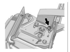
Your vehicle has a remote negative (-) ground location, as shown in the illustration. It is located on the left side of the engine compartment. See Engine Compartment Overview on page 10-6. You should always use this remote ground location, instead of the terminal on the battery.
